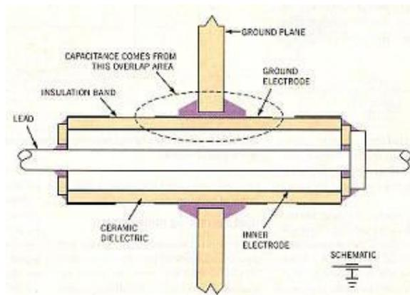
Capacitive filters can be created in a variety of ways including the use of discrete capacitors or layered ceramic components.
