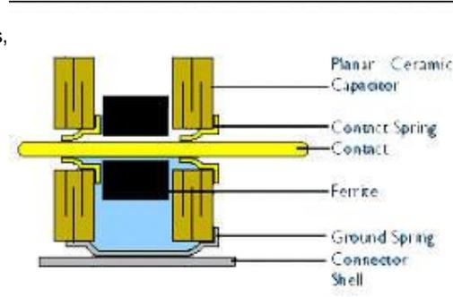
Some applications that require relatively low levels of filtering may use simple blocks of ferrite attached to the back end of a connector. These were particularly popular within the personal computer market where price pressures would not permit higher performance solutions. They are often used to provide a bit of extra margin when a particular device may be close to an emission limit.
