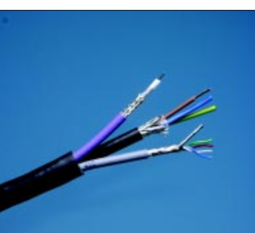
The BD CMQVP hybrid monitor cable from Bryant Broadcast and Data Communications incorporates a screened 3-core, 6A power supply cable; an SDI video cable; and lap screened audio star quad — all in a single jacket.
